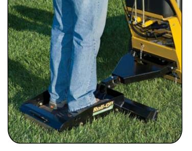
responsiveness. The operator-presence safety system (yet another soon-to-be-patented Hustler exclusive) requires no squeezing, no gripping to engage. Because the TrimStar is first and last a Hustler, expect a blade spindle proven amid 35 years of durable, reliable service. Expect bearings that refuse to waste horsepower
