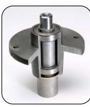
Best blade-spindle design in the industry! Sealed bearings require minimal maintenance, less horse power, and generate less heat. Grease every 500 hours! 3-year warranty on bearings.
